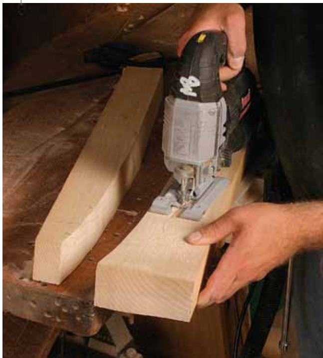
Cut curves without a bandsaw. A jigsaw can often handle the task, even on thick stock like this 8/4 maple. On stock this thick, premium blades are worth the extra cost. Cheaper versions can deflect, creating an out-of-square cut.
